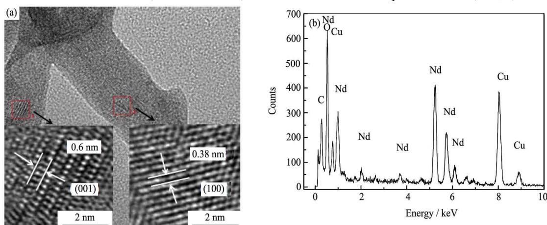
Fig. 1 HRTEM image (a) and EDS picture (b) of hexagonal phase of Nd<sub>2</sub>O<sub>3</sub> nanorods
