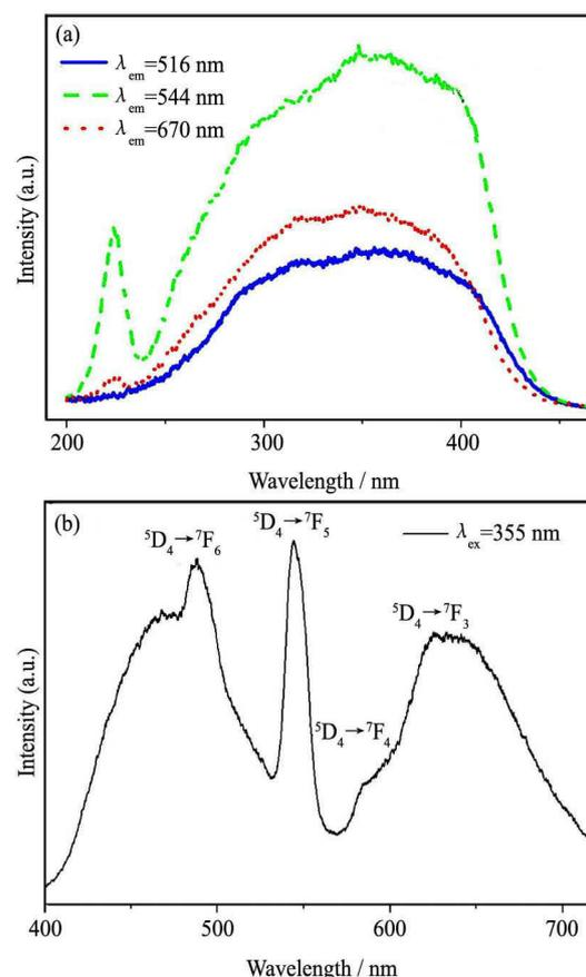
Fig. 2 PLE and PL spectra of the sample  $\text{KCaPO}_4:7\%\text{Eu}^{2+}, 7\%\text{Tb}^{3+}, 2\%\text{Mn}^{2+}$  respectively
