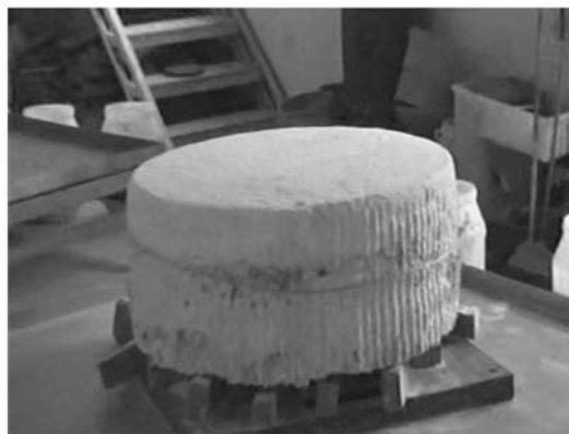
Fig. 1 As-grown YSZ ingot with a diameter of 100 cm and a height of 80 cm
