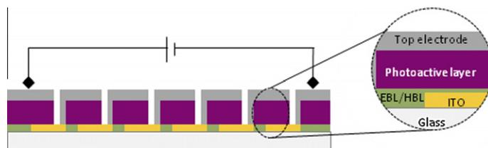
Fig. 1. Cross section of a series-connected module where the patterning required for each layer and the interconnections among the subcells can be seen.
