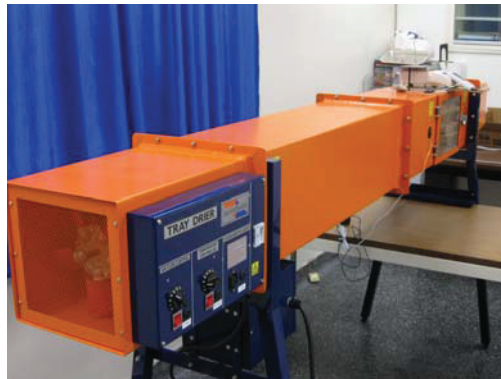
Fig. 2. Armfield Model UOP-8 laboratory-scale tray dryer
