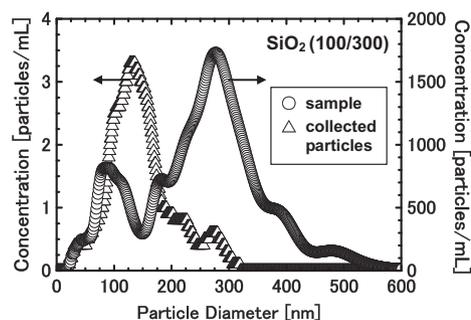
Fig. 2. Concentration of particles contained in original sample mixture of SiO<sub>2</sub> (100 and 300 nm) and of collected particles.
