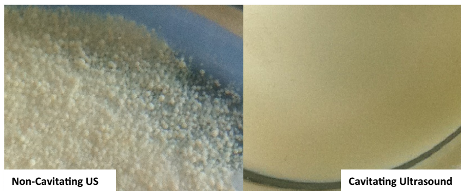
Fig. 1. Effect of non-cavitating and cavitating US on immobilized enzymes.
