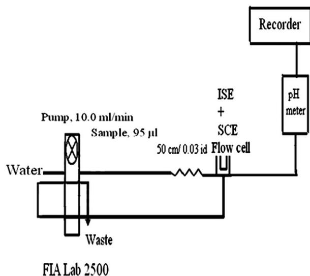
Fig. 1. Schematic diagram of the flow injection system used in measurements.
