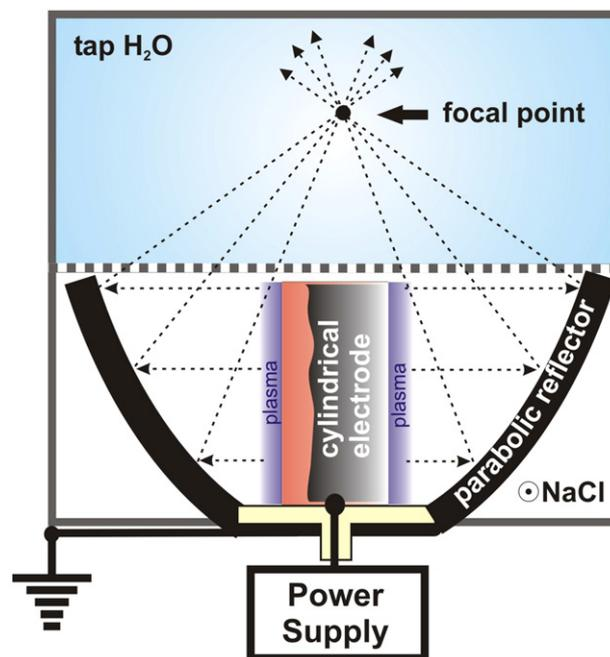
Fig. 1. Scheme of shock wave generator.
