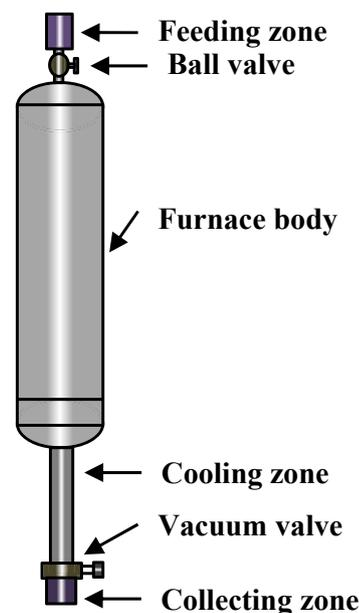
**Fig. 1** – Schematic diagram of vertical high-temperature tube furnace for fabricating HGMs using the dried gel method.
