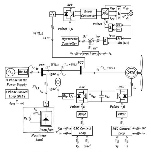
Fig. 1 – Overall circuit diagram configuration of hybrid wind solar energy system.
