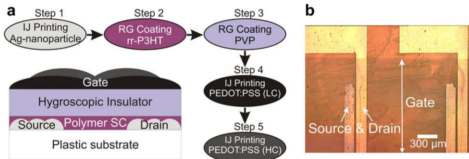
**Fig. 1.** (a) A five-step process flow for the fabrication of all-printed low-voltage organic transistors and a schematic image of a cross section of the transistor. Semiconductor is denoted as SC, while low- and high-conductive is denoted as LC and HC and (b) An optical microscope top-view picture of two all-printed devices.
