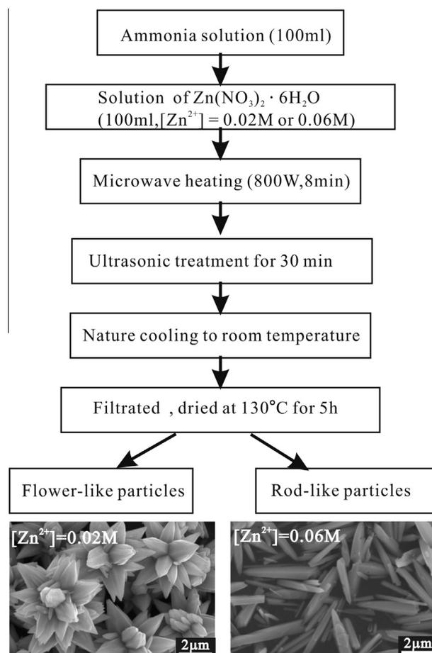
Fig. 1. Flow-charts representing the experiment procedure for the fabrication of ZnO particles with flower- and rod-like morphologies.  $[Zn^{2+}]$  represents the concentration of zinc ion in solution.
