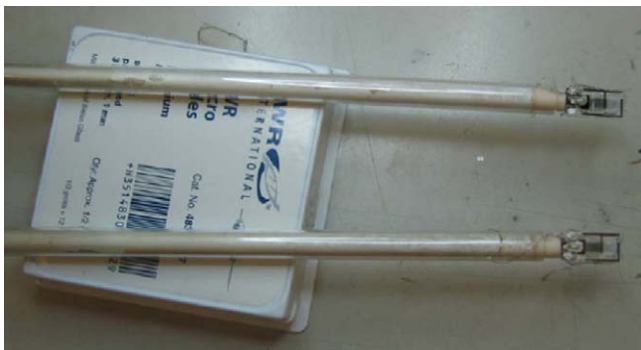
Fig. 1. Gas sensor prototypes mounted on \text{Al}_2\text{O}_3 holders. (Note: The illustrated sensors resemble the ones used in this study.)
