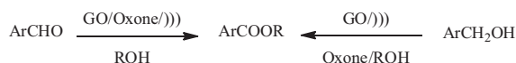
Scheme 1. Sonochemical direct oxidative esterification of aldehydes and benzyl alcohols using GO/Oxone in alcoholic solvent.
