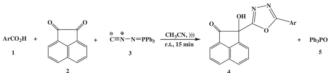
**Scheme 1.** Synthesis of disubstituted 1,3,4-oxadiazole derivatives under ultrasound irradiation.
