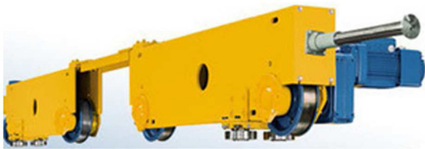
Fig. 1 – Cart with horizontal offset-adjusting wheels.
