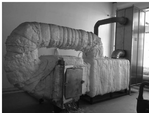
Fig. 2 – General view of the research & demonstration preheat catalytic reaction reactor apparatus.
