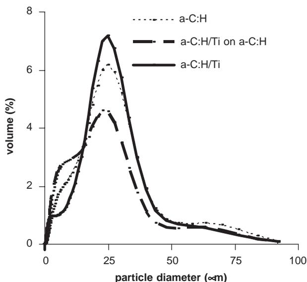
Fig. 1. Particle size distribution counted using a Beckman Coulter.
