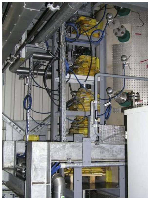
Fig. 2 – Detectors installed at the reactor (encased in the yellow lead bricks) [6].
