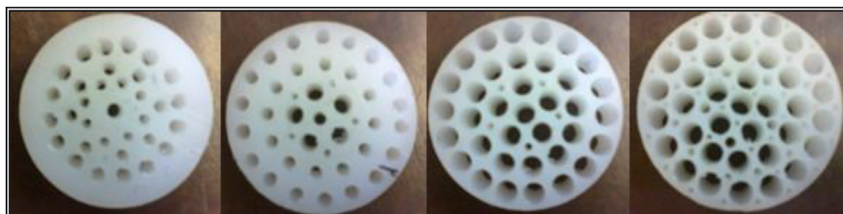
Fig. 1 – Polyethylene phantoms which are used to model void fractions in homogenous flow.
