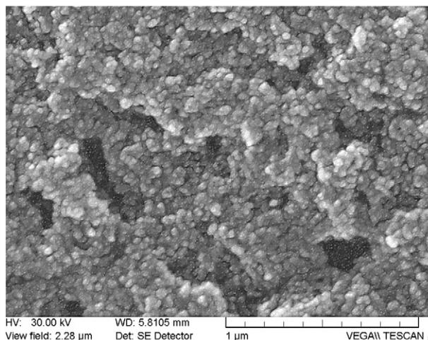
Image 1. SEM recording of  $\text{Fe}_3\text{O}_4/\text{T}$  core/shell systems.
