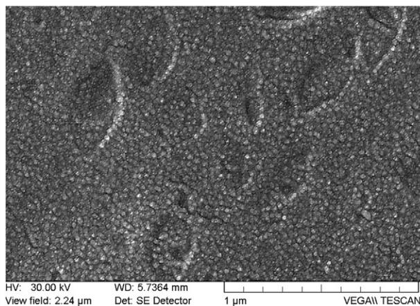
Image 2. SEM recording of  $\text{Fe}_3\text{O}_4/\text{S}$  core/shell systems.
