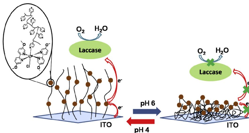
**Scheme 1.** The pH-switchable bioelectrocatalytic electrode for oxygen reduction biocatalyzed by laccase and mediated by the redox-polymer brush bound to the electrode surface.
