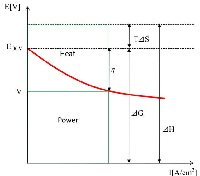
Fig. 1 – Energy balance in I–V characteristics of general SOFC.
