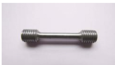
Fig. 2 – Geometry of the tensile specimen.
