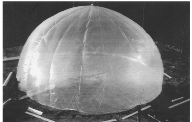
Fig. 1. The hemispherical balloon with hydrogen–air mixture, R_0 = 10 \text{ m} .
