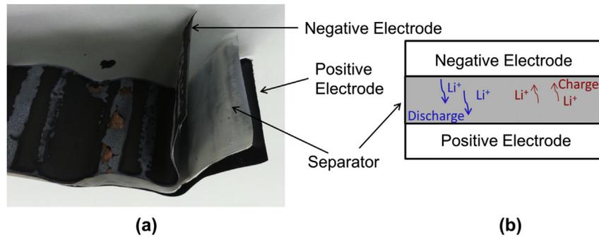
Fig. 1. (a) Image of the electrode-separator roll in a Li-ion cell; (b) Schematic of various layers in the assembly.
