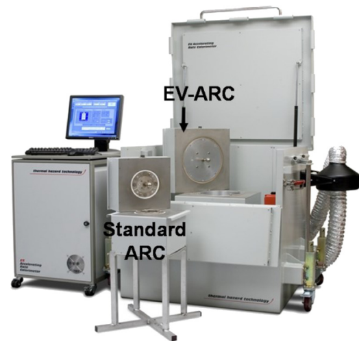
Fig. 1. The illustration of the es-ARC with double systems made by the THT.
