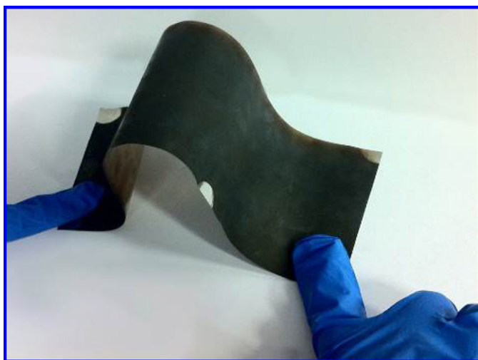
Fig. 1. Solution precursor plasma deposited flexible \text{Co}_3\text{O}_4 electrode on a stainless steel sheet (SS304) current collector.
