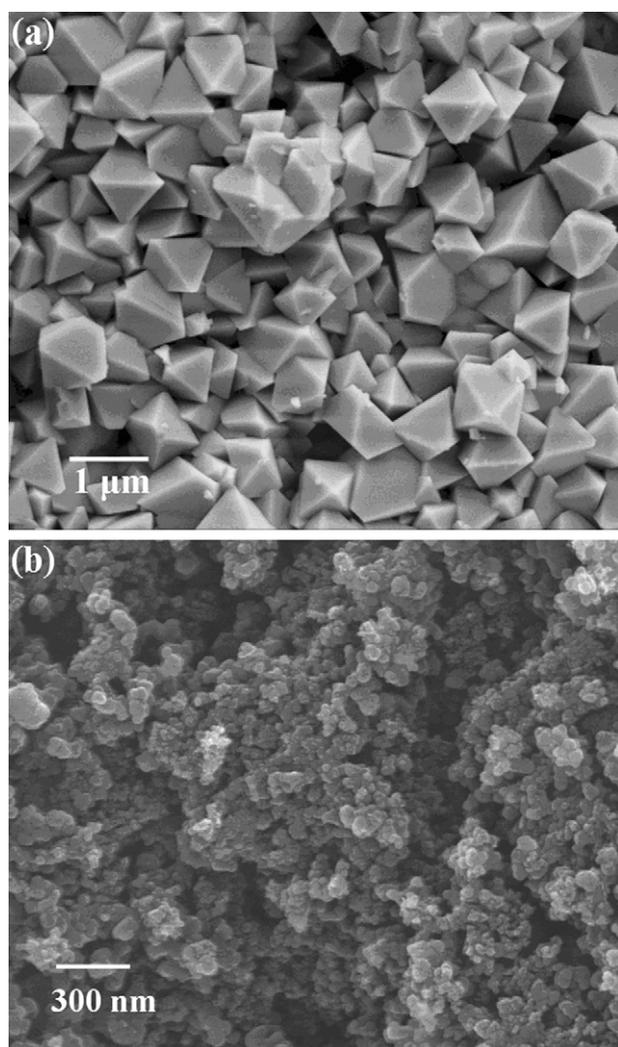
Fig. 1. SEM micrographs of (a)  $\text{LiMn}_2\text{O}_4$  and (b)  $\text{MnFe}_2\text{O}_4$ @C composite.
