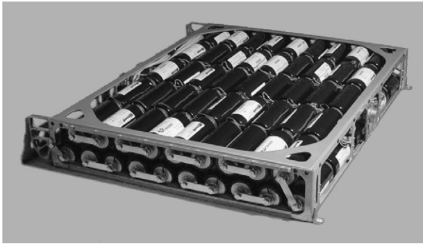
Fig. 1. Picture of the 250 V supercapacitor module for the HY-LIGHT hybrid vehicle.
