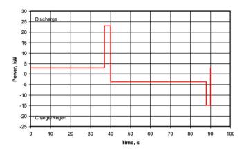
**Fig. 3.** Charge-sustaining cycling profile [19]. The power levels given on the vertical axis are divided by the BSF to yield the actual power levels used to test a given battery. The unscaled profile removes 50 Wh during the discharge portion of the cycle; the regen portion charges the battery with 46.2 Wh of energy, producing a net removal of 3.8 Wh.
