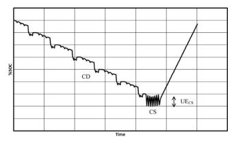
**Fig. 1.** Schematic showing the two PHEV operating modes, charge-depleting and charge-sustaining (after Ref. [19]). In charge-depleting mode, the internal-combustion engine is not used; energy from the battery alone powers the vehicle. The charge-sustaining mode is similar to that of the HEV; the power from the battery supplements that from the engine. The abbreviation, UE<sub>CS</sub>, shown in the figure, is the SOC window from which the usable energy in CS mode is based.
