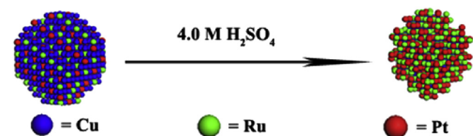
Scheme 1. Illustration of PtRuCu 6 -A/C by chemical corrosion.
