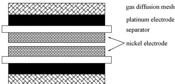
Fig. 1. Schematic diagram of an electrode stack.
