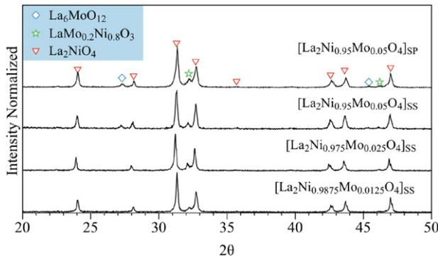
**Fig. 1.** Diffractograms of  $\text{La}_2\text{Ni}_{1-x}\text{Mo}_x\text{O}_{4+\delta}$  with  $x = 0.0125, 0.025,$  and  $0.05$ . All SS-samples are sintered at  $1300^\circ\text{C}$  while SP-sample is sintered at  $1400^\circ\text{C}$ . The presence of the major phase is compared with the characteristic reflections for tetragonal  $\text{La}_2\text{NiO}_4$ .
