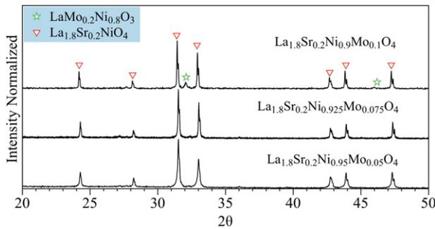
**Fig. 2.** XRD-data for  $\text{La}_{1.8}\text{Sr}_{0.2}\text{Ni}_{1-x}\text{Mo}_x\text{O}_{4+\delta}$  (SS-samples) with  $x = 0.05, 0.075$  and  $0.1$ . All samples are sintered at  $1300^\circ\text{C}$ . The major LN phase is compared with the characteristic reflections for  $\text{La}_{1.8}\text{Sr}_{0.2}\text{NiO}_4$ .
