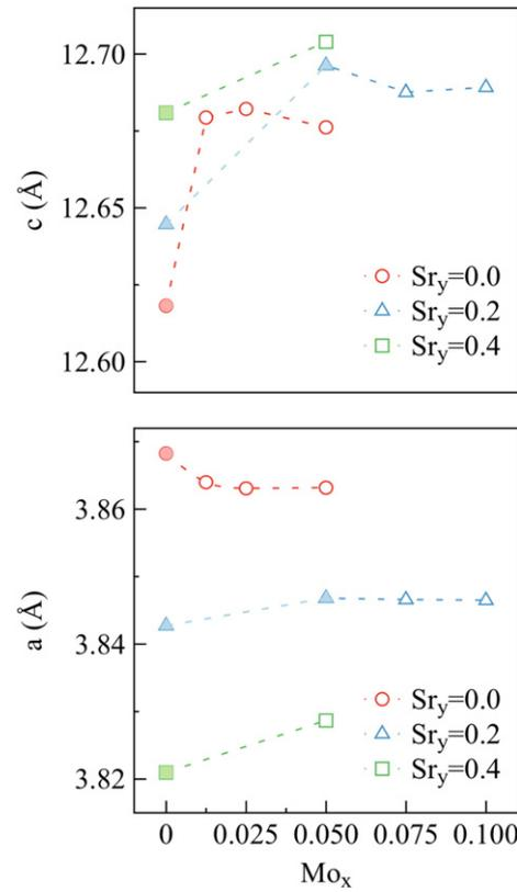
**Fig. 3.** Variation in cell parameter for  $\text{La}_2 - y\text{Sr}_y\text{Ni}_{1-x}\text{Mo}_x\text{O}_{4+\delta}$  with Mo-content for compositions with 0.0, 0.2 and 0.4 Sr. Cell parameters for  $\text{La}_2\text{NiO}_4$  is taken from [14]. Samples are heat treated at  $T = 1300^\circ\text{C}$ . Filled symbols indicate single phase while open symbols indicate the presence of secondary phases. Magnitude of error will typically be within the size of the symbols given in the figures.
