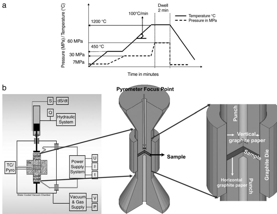
Fig. 1. (a): Sintering cycle used in PECS for sintering electrolyte and half cells. (b): Schematic set-up of die with powder loading as used in PECS.
