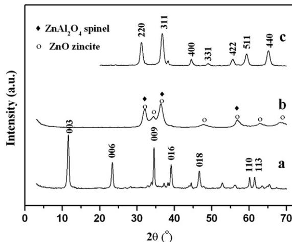
Fig. 1. Powder XRD patterns of (a) the ZnAl-LDH precursor, (b) ZnAl-LDH calcined at 700 °C for 2 h, and (c)  $\text{ZnAl}_2\text{O}_4$ .
