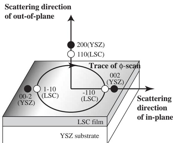
Fig. 1. Schematic illustration of X-ray scattering geometry.
