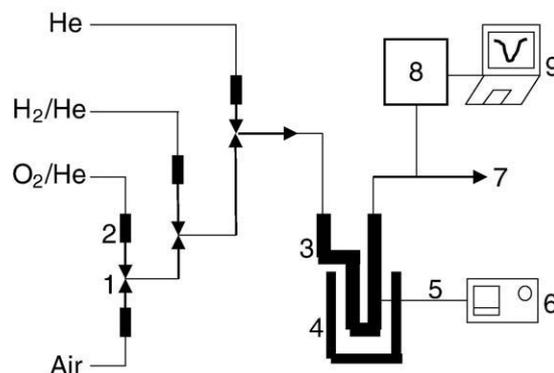
**Fig. 1.** TPO experimental setup. 1—Three-way valve; 2—Mass flow controller; 3—U-type quartz reactor; 4—Electric furnace; 5— Thermal couple; 6—Temperature controller; 7—Exhaust gas; 8—Mass spectrograph; 9—Recorder.
