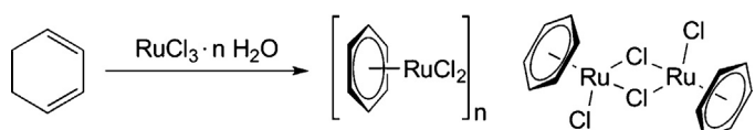
Fig. 2. Synthesis of benzene ruthenium dichloride considered to be a polymer [10], until its dimeric nature, [(\eta^6\text{-C}_6\text{H}_6)\text{Ru}(\mu_2\text{-Cl})\text{Cl}]_2 , was established [11–14].
