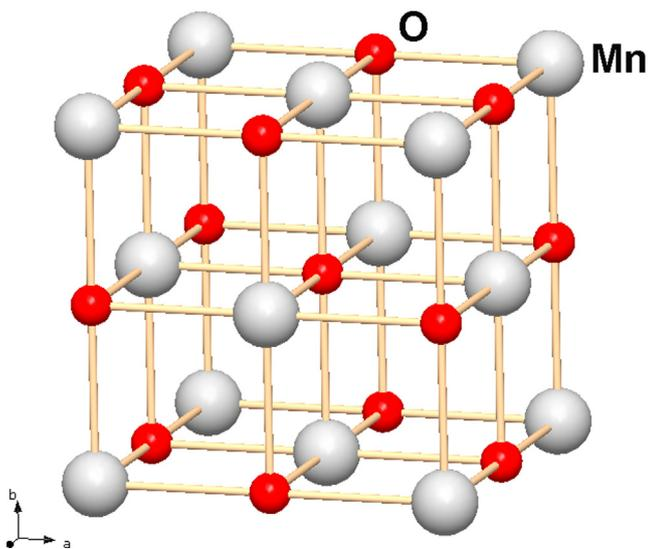
Fig. 1. Structure of the cubic Mn(II) oxide.
