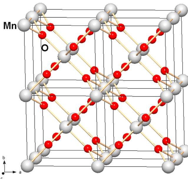
Fig. 2. Tunnel structure of pyrolusite with channels along *c*.
