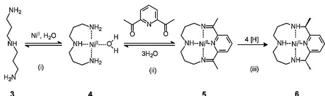
**Scheme 2.** The nickel(II) template synthesis of CR (5) and CRH (6) tetra-aza-macrocyclic complexes. The cyclization step (ii) involves the reversible Schiff base condensation of the carbonyl groups of 2,6-diacetylpyridine with the –NH<sub>2</sub> groups of the triamine 3, preoriented through coordination to the metal.
