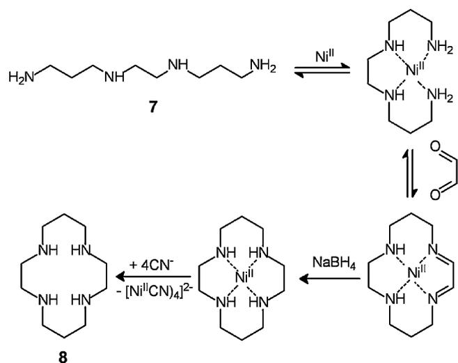
**Scheme 3.** The nickel(II) template synthesis of cyclam, 1,4,8,11-tetra-azacyclotetradecane (8) [10]. The cyclization step involves the reversible Schiff base condensation of the carbonyl groups of glyoxal with the –NH<sub>2</sub> groups of the linear tetramine 7, preoriented through coordination to the metal.
