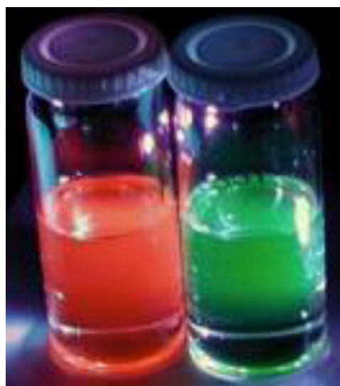
Fig. 2. Digital picture of CdSe colloidal QDs of different sizes prepared at ICIQ illuminated with UV light.
