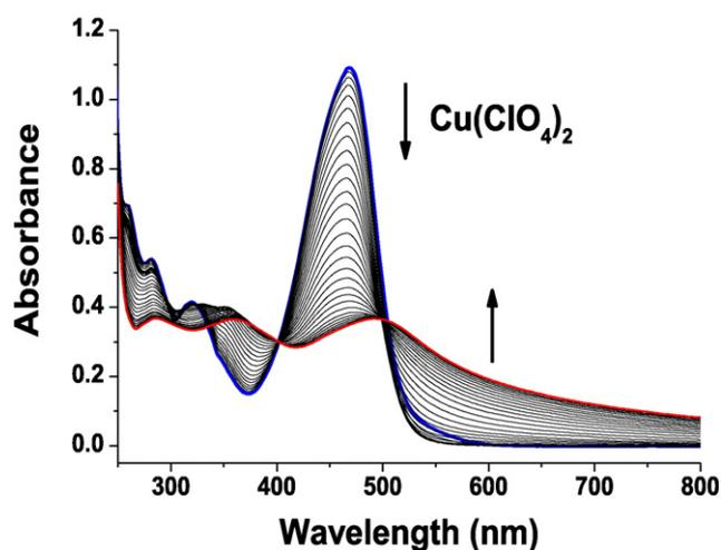
Fig. 1. UV-vis spectra of **L** (20  $\mu\text{M}$ ) in  $\text{CH}_3\text{CN:H}_2\text{O}$  (4:1, v/v) solution upon addition of increasing concentrations of  $\text{Cu}(\text{ClO}_4)_2$ .
