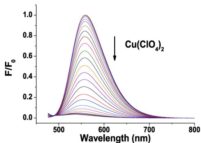
Fig. 2. Fluorescence emission spectra of **L** (20  $\mu\text{M}$ ) in  $\text{CH}_3\text{CN:H}_2\text{O}$  (4:1, v/v) solution upon addition of increasing concentrations of  $\text{Cu}(\text{ClO}_4)_2$  with an excitation wavelength at 466 nm.
