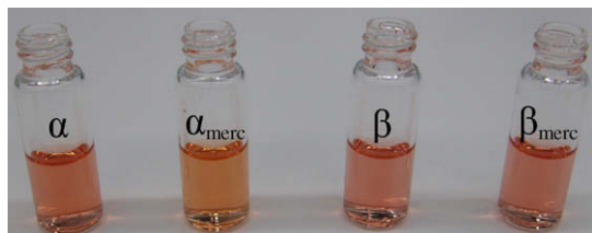
Fig. 2. Digital picture of four samples containing different stereoisomers in the presence and absence of mercury chloride (1 ppm) added from a 10^{-3} \text{ M} ethanolic-based \text{HgCl}_2 stock solution).
