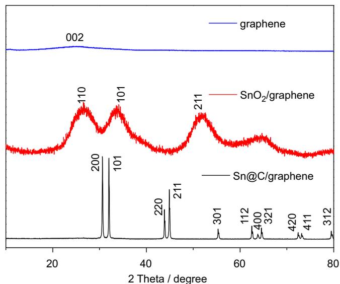
Fig. 1. XRD patterns of graphene, SnO<sub>2</sub>/graphene and the as-prepared Sn@C/graphene.
