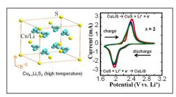
Tuning Li content in  $Cu_{4-x}Li_xS_2/Li$  half-cells to maintain a Cu/Li ratio equal to unity affords maximum capacity and high stability of the charge–discharge process.
