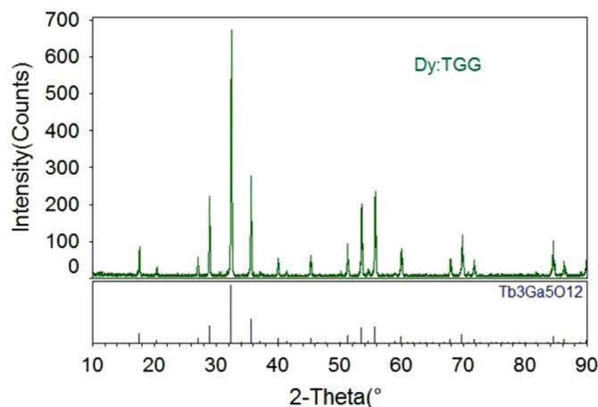
Fig. 2. X-ray powder diffraction patterns of the  $\text{Dy}^{3+}$ -TGG.
