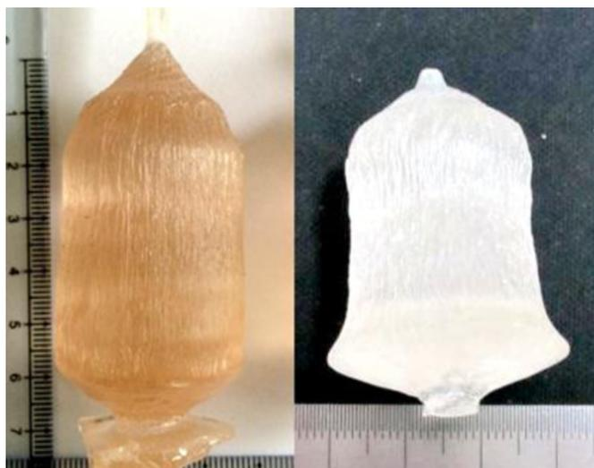
Fig. 1. The picture of as-grown crystals by the Cz method. The left is the  $\text{Dy}^{3+}$ -TGG and the right is the pure TGG.
