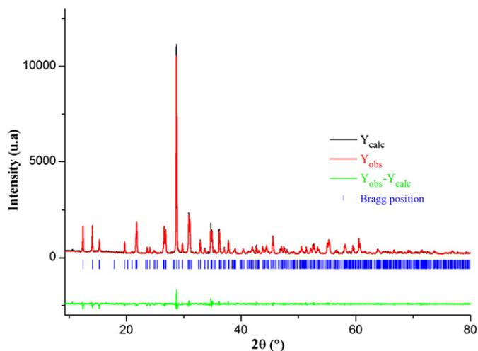
Fig. 1. The powder X-ray diagram of  $\text{KCuFe}(\text{PO}_4)_2$ .
