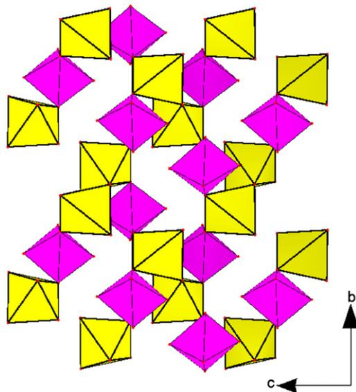
Fig. 3. The  $\text{Cu/Fe/O}$  sub-network forming sheet parallel to the  $bc$  plane. Legend:  $\text{CuO}_5$  polyhedra=yellow and  $\text{FeO}_6$  polyhedra=purple. (For interpretation of the references to color in this figure legend, the reader is referred to the web version of this article.)
