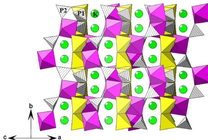
Fig. 2. A projection along the  $[010]$  direction of the structure showing the six-edged tunnels, occupied by the  $\text{K}^+$  ions. Legend:  $\text{CuO}_5$  polyhedra=yellow;  $\text{PO}_4$  tetrahedra=hatched;  $\text{FeO}_6$  polyhedra=purple; and  $\text{K}^+$  cations=green circles. (For interpretation of the references to color in this figure legend, the reader is referred to the web version of this article.)
