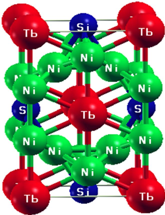
Fig. 1. The structure of TbNi<sub>4</sub>Si compound.
