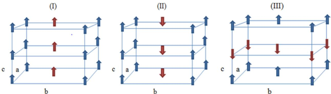
Fig. 2. The three studied configurations (I) ferromagnetic configuration (II) type (A) antiferromagnetic configuration (III) type (B) antiferromagnetic configuration.
